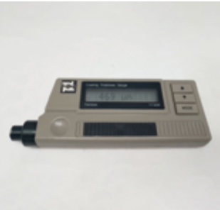
Coating thickness gauge 合金层厚度检测
